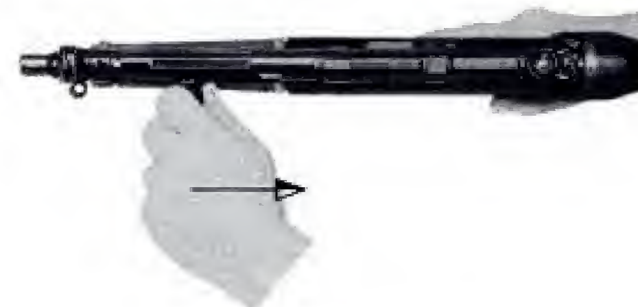
Fig. 29 Retracting the cocking lever
